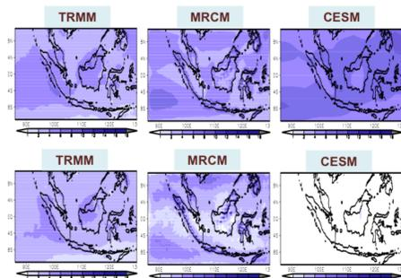
• In contrast to the similar behavior of total precipitation, MRCM and CESM show the different details such as partitioning of convective and large-scale precipitation.
